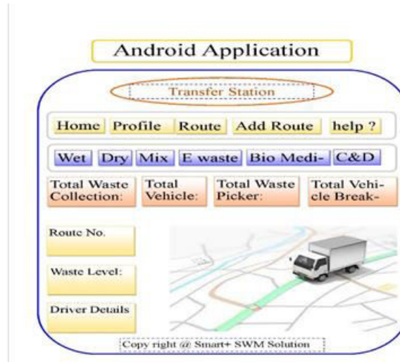
Figure 5: Transfer Station Interface
